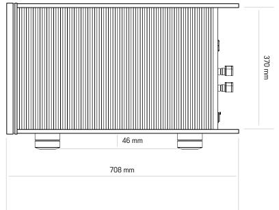
**Material:** Aluminium for body parts and heat sinks **Dimensions (H x W x D):** 445 x 505 x 708 (mm) **Weight:** 126Kg
